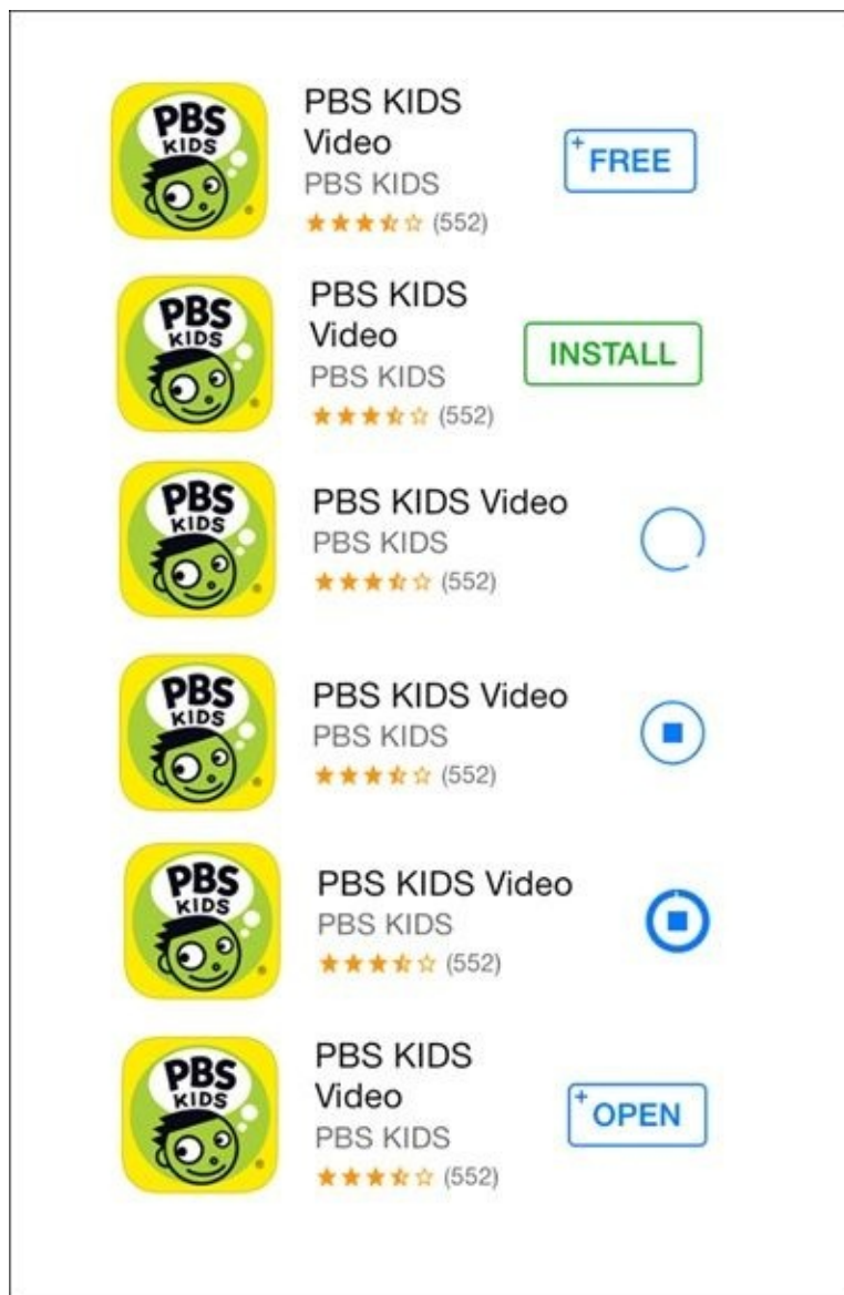
Figure 5-29. App Store for iOS: Multi-State Buttons show buy, install, progress, and open options
